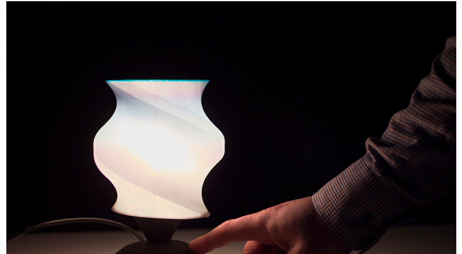
Conductive plastic-based lamp with tactile-switch manufactured by 3D printing
